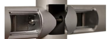
Kee Lite<sup>®</sup> Smooth components utilize a stainless steel cap screw for thru-bolt connection and expanding internal fingers to create the most rigid connection available for a smooth handrail system.
