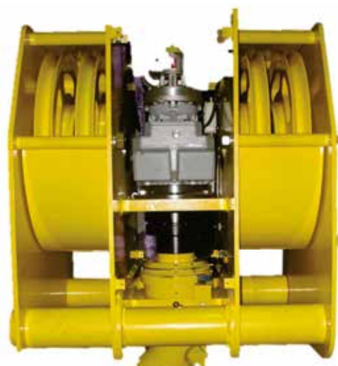
Hook driving with electromagnetic latch
