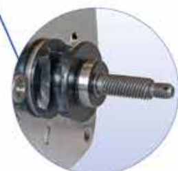
Ball bearing mounted sprocket shaft
