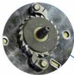
Safety brake with two stainless steel pawls
